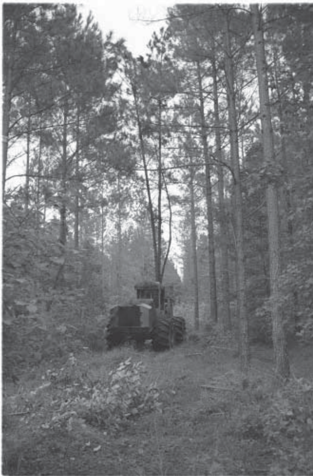
Figure 1. Feller-buncher carrying out a second thinning in an 18-year-old loblolly pine plantation just north of Greenville, NC.
