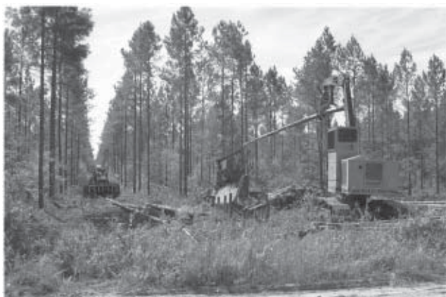
Figure 5. Tigercat 245 tracked loader pulling a stem through the static delimber.
