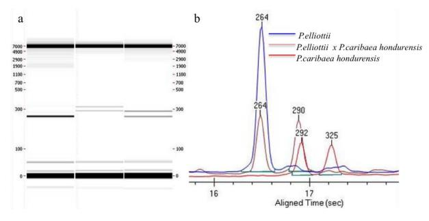
*Figure 3*: Fragment analysis of a SSR marker in the hybrid Pinus elliottii var. elliottii x Pinus caribaea var. hondurensis and in the species Pinus elliottii var. elliottii and Pinus caribaea var. hondurensis, using an automated electrophoresis system. (a) Example of a virtual gel image and (b) an electropherogram of the three biological samples.
