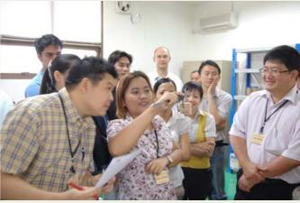
Photo: Courtesy of Walailak University Measuring the thickness of a particleboard sample after soaking it 24 hours in water
