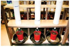
Fig 1. Soil in nursery pots is treated with various rates of PAM and irrigated with a zoospore solution or just DI water. Leachate is collected below the pot and the propagules are counted.
