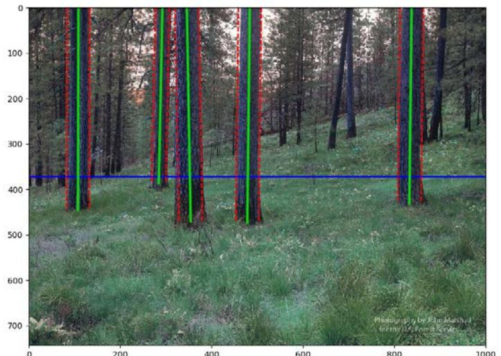
*A 3D machine vision technology developed to detect and measure tree characteristics real-time during thinning operations. (Credit: Lucas Wells, Oregon State University)*
