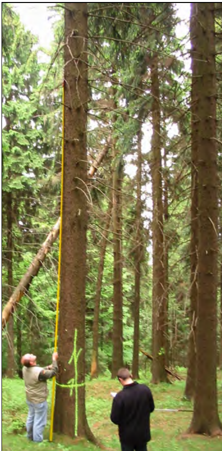
Figure 3: Measuring branch diameters according to the 'Tharandter Erdstammethode' ('Tharandter Butt Log method')
