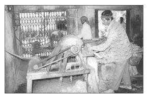
Figure 5—Society members decorticating Agave leaves on motorized decorticating machines at Kolchur Centre, Jagdalpur.
