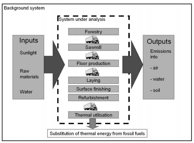
Figure 1-Life cycle of wood floor coverings.
