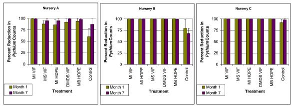
**Figure 1.** Percent reduction in *Pythium* species counts from dilution plating of fumiganttreated soil at three forest tree nurseries. MI = methyl iodide, MS = metam sodium, DMDS = dimethyl disulfide, MB = methyl bromide, VIF = virtually impermeable film, HDPE = high density polyethylene.
