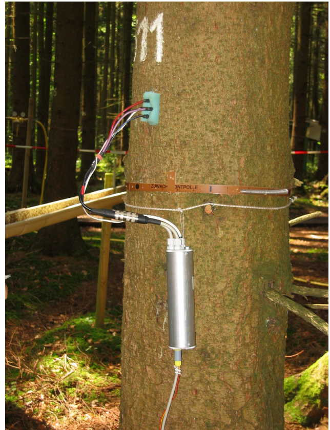
Sap-flow measurements for the calculation of crown-level stomatal ozone flux in Norway spruce
