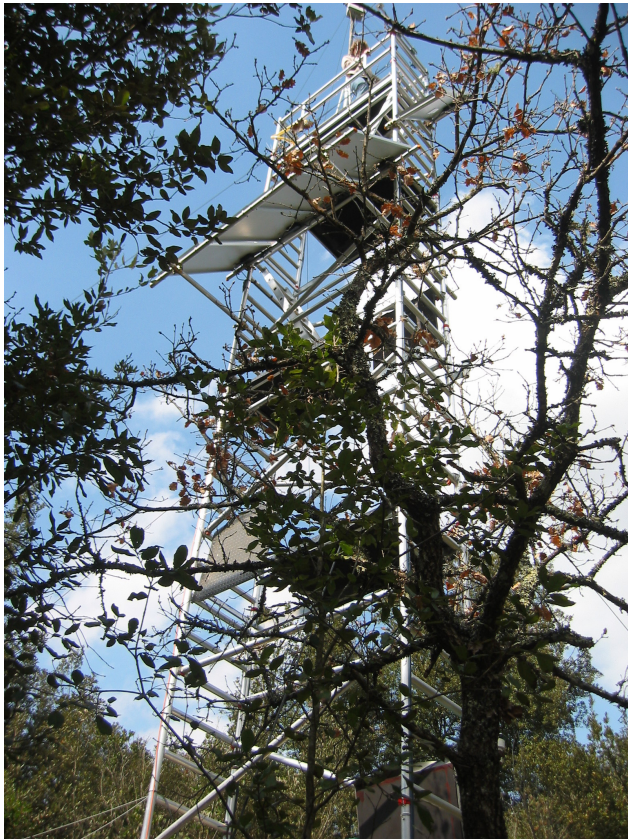
Eddy-correlation tower for measuring canopy-level ozone flux in a Mediterranean forest
