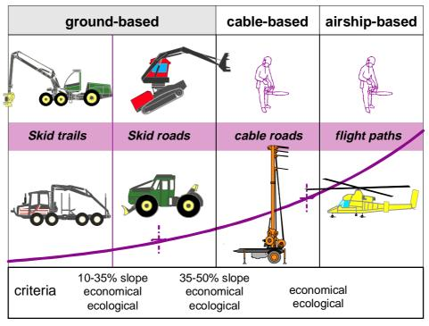
Fig. 1Basic harvesting system concepts. Off-road transportation technology is<br/>decisive for the layout of road networks and harvest units.
