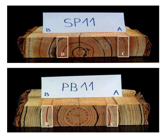
Fig. 2. Location of the battens in a central plank (85mm thick). Tree SP11 is more than 60 years old whilst tree PB11 is around 40y.o.
