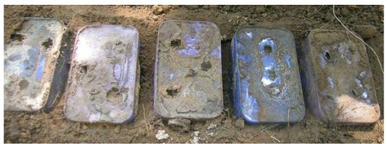
Figure1: Set up of field termite test
