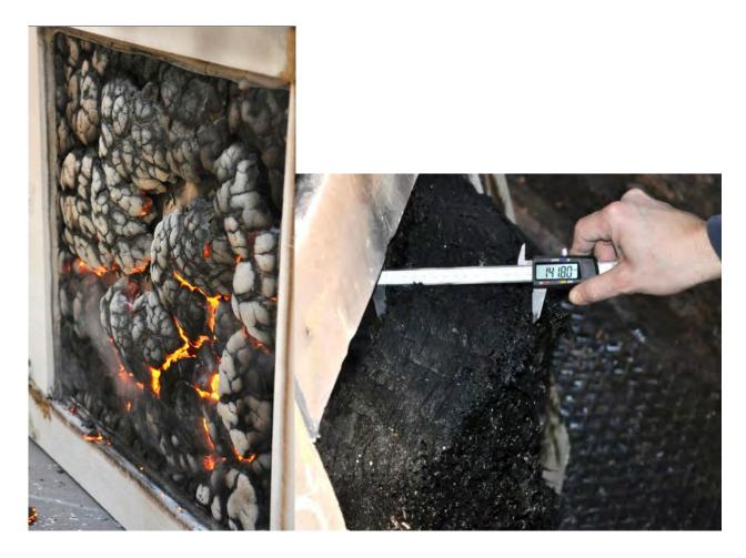
Figure 7: Foaming of 50 WB panel (left) and foam thickness of 100 WW (right)
