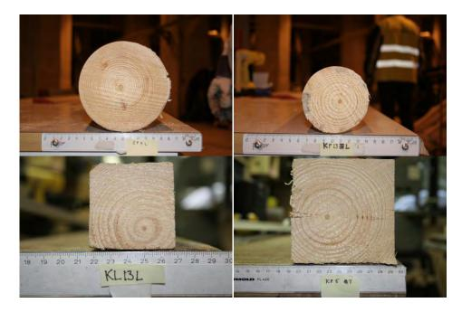
Figure 1: Examples of the round (80 and 120 mm) and square (50×50 mm and 100×100 mm) post specimens.
