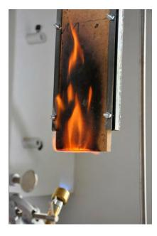
Figure 1: Procedure of small flame test
