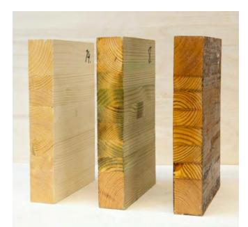
Figure 1: Examples of tested 44x200x200 mm glulam specimens. From the left: untreated, CCimpregnated, and pine oil impregnated. The material from small sized timber was mainly sapwood which can be seen as high penetration of preservative liquid in the inner lamellae of the CC-impregnated specimen, whereas virtually no preservative has penetrated in the surface lamellae that were made of larger logs with higher proportion of heartwood. (Photo: Erkki Oksanen, Metla)
