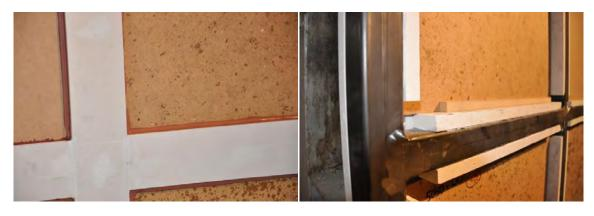
Figure 2: Fire test preparation (left: flame exposed, right: flame averted)
