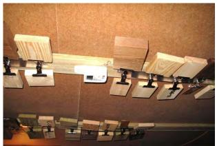
Figure 1. Test pieces and the data logger mounted on the blind floor.
